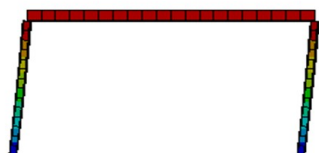
Fig. 7 Deformation of bare frame
